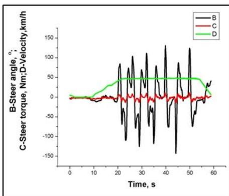
Figure 3 Time history of registered input values during the overtaking test
