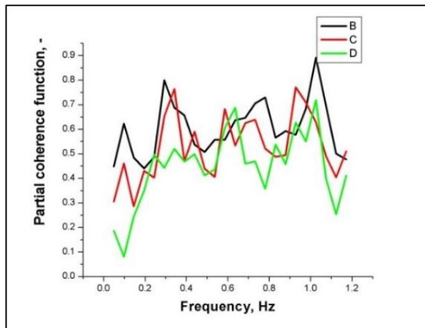
Figure 19 Partial coherence function: yaw – steering wheel angle (B), torque at steering wheel with excluded influence of steering wheel angle (C) and velocity with excluded influence of angle and torque at steering wheel (D), in rectilinear driving test
