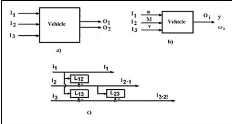
Figure 17 Scheme of a system with three input and two output sizes (legend:  $I_1$ - $I_3$  present input excitation values ( $\alpha$ ,  $M$ ,  $v$ ), and  $O_1$ - $O_2$  registered lateral accelerations and yaw ( $a_y$ ,  $\omega_z$ ))
