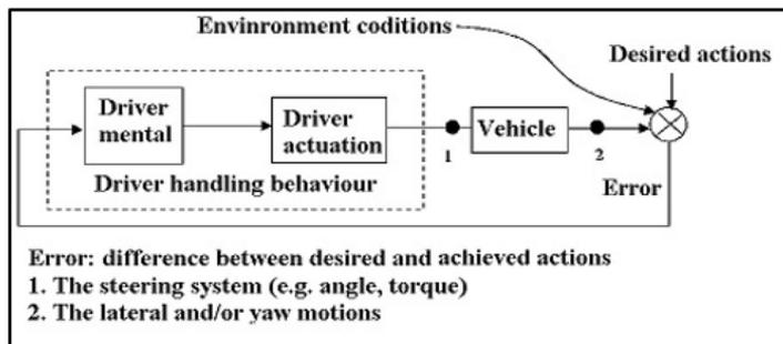
Figure 1 Control system: Driver-Vehicle-Environment
