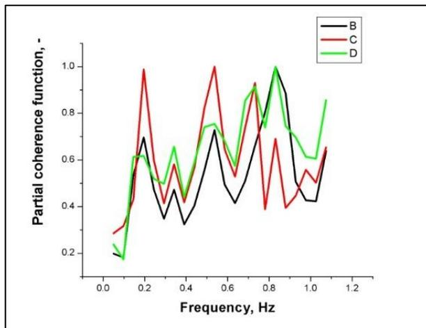
Figure 23 Partial coherence function: yaw – steering wheel angle (B), torque at steering wheel with excluded influence of steering wheel angle (C) and vehicle velocity with excluded influence of angle and torque at steering wheel (D) during overtaking test
