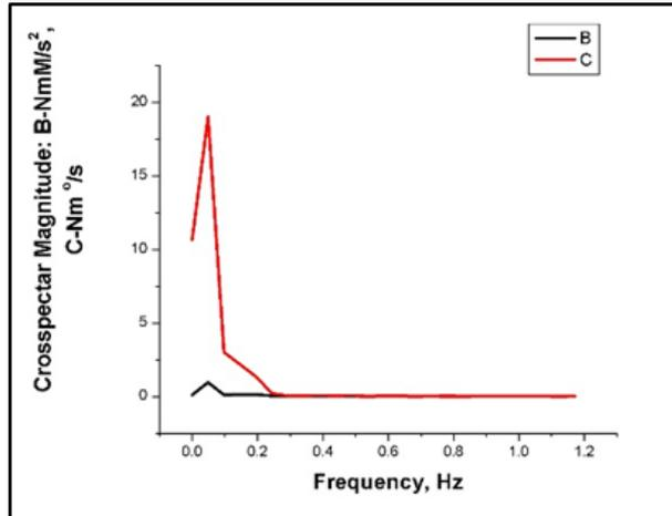
Figure 15 Cros-spectra: Torque at steering wheel – lateral acceleration, Torque at steering wheel -yaw during DLC test
