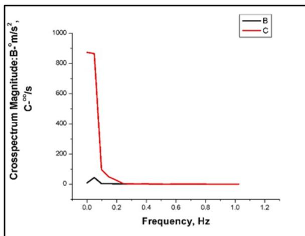
Figure 14 Cross-spectra: steering wheel angle – lateral acceleration, steering wheel angle -yaw during DLC test
