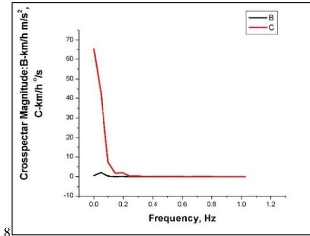
Figure 16 Cros-spectra: Velocity – lateral acceleration, Velocity -yaw during DLC test
