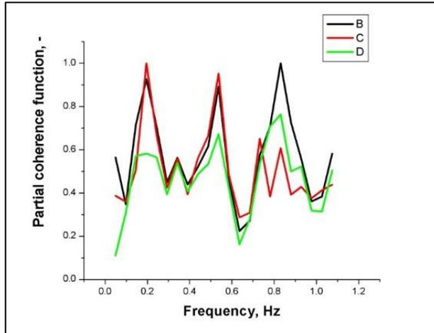
Figure 22 Partial coherence function: lateral acceleration – steering wheel angle (B), torque at steering wheel with excluded influence of steering wheel angle (C) and vehicle velocity with excluded influence of angle and torque at steering wheel (D) during overtaking test
