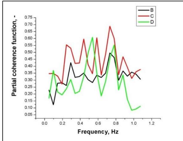
Figure 18 Partial coherence function: lateral acceleration – steering wheel angle(B), torque at steering wheel with the excluded influence of the steering wheel (C) and velocity with excluded influence of angle and torque at steering wheel (D), in rectilinear drive test
