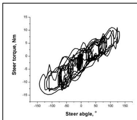
Figure 4 Couple: Steer angle – Torque at steering wheel during overtaking test
