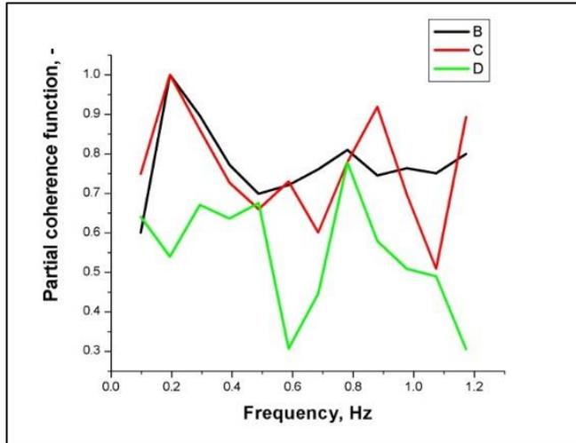
Figure 21 Partial coherence function: yaw – steering wheel angle (B), torque at steering wheel with excluded influence of steering wheel angle (C) and velocity with excluded influence of angle and torque at steering wheel (D) during DLC test
