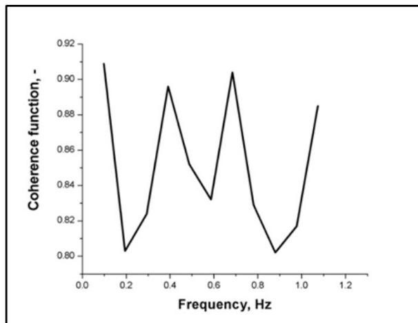
Figure 13 Coherence: Torque at steering wheel – vehicle velocity during overtaking test
