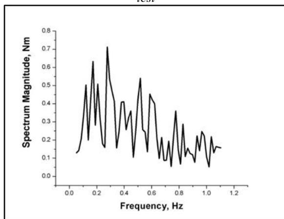
Figure 9 The magnitude of the torque amplitude spectrum at the steering wheel during the overtaking test
