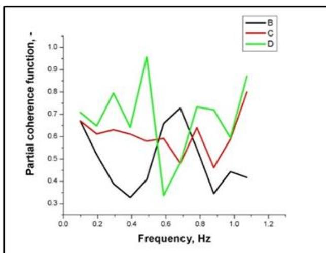
Figure 20 Partial coherence function: lateral acceleration – steering wheel angle (B), torque at steering wheel with excluded influence of steering wheel angle (C) and velocity with excluded influence of angle and torque at steering wheel (D) during DLC test
