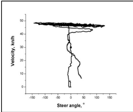
Figure 5 Couple: Angle of steering wheel – vehicle velocity during overtaking test
