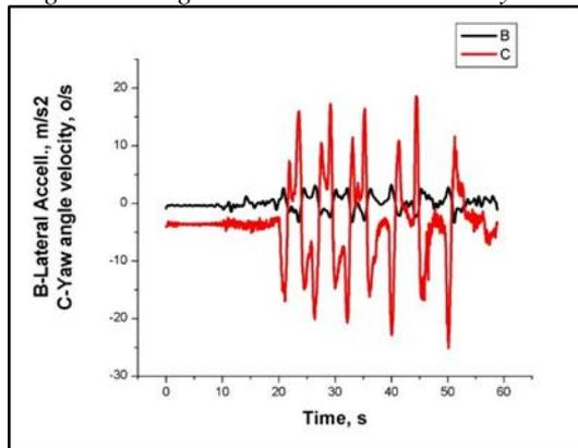
Figure 7 Lateral acceleration and angular yaw velocity of the truck during the overtaking test
