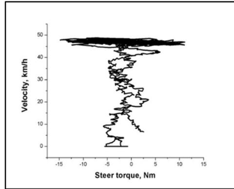
Figure 6 Couple: Torque to steering wheel – vehicle velocity during overtaking test
