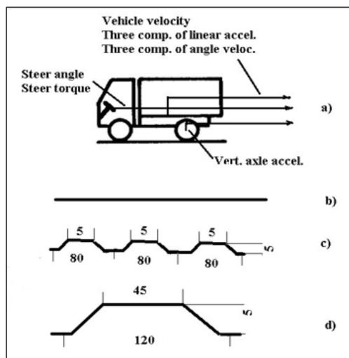
Figure 2 a) Diagram of measuring points during the FAP 1118 vehicle behavior test b) sketch of overtaking test; c), sketch of DLC test; d) rectilinear driving- dimensions, [m]
