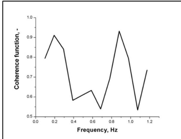
Figure 11 Coherence: Angle of steering wheel– torque at steering wheel during overtaking test
