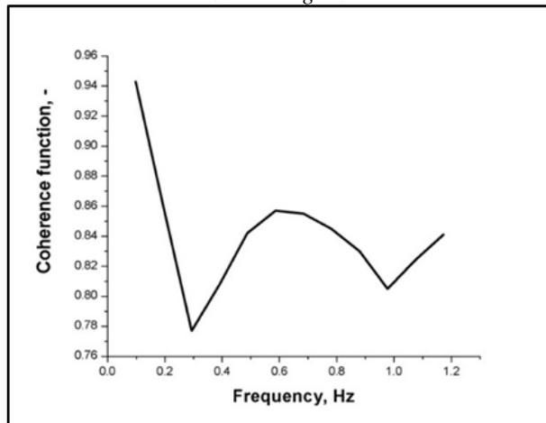
Figure 12 Coherence: Angle of steering wheel – vehicle velocity during overtaking test
