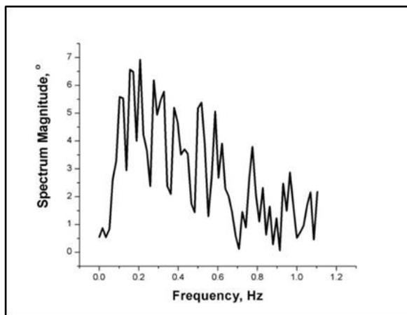
Figure 8 The magnitude of the steering angle amplitude spectrum during the overtaking test
